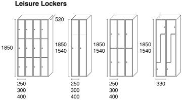
Single unit up to 3 tier Max carcass h/w/d = 2000/600/800mm
