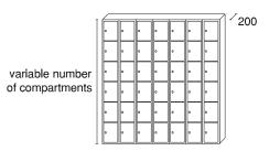
Max carcass height 2000mm Glass doors min h/w/d = 280/250/200mm
