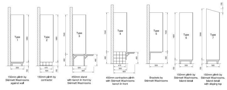
Supporting stands can have plinth infill panels on request. All locker constructions are available with either flat or sloping tops.
